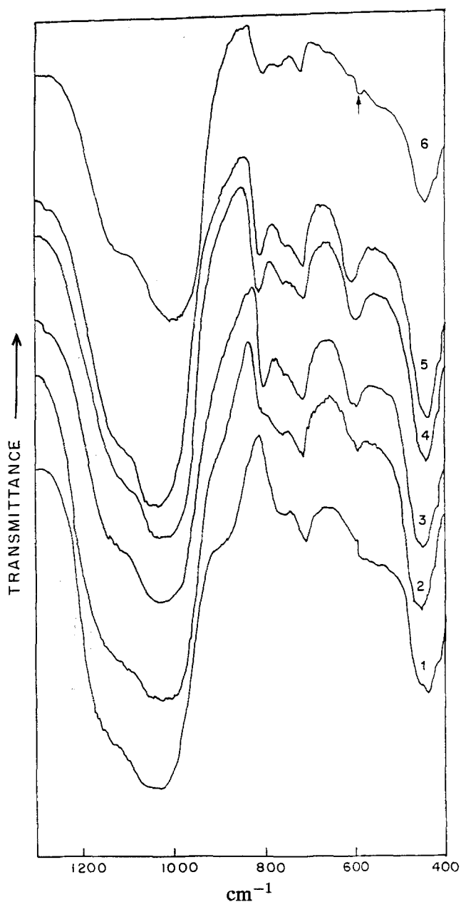
Fig. 4. Framework IR spectra of samples with different degree of crystallinity. Al-omega (1) 0%, (2) 26%, (3) 72%, (4) 93%, (5) 100% and (6) 100% Ga-omega.
